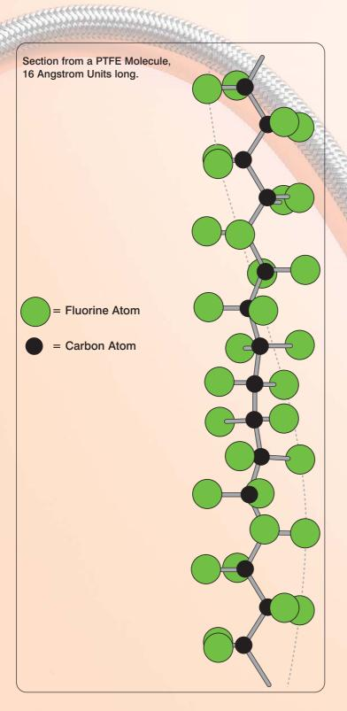
PTFE, or Polytetrafluoroethylene, comprises long-chain molecules of carbon atoms, each linked to two fluorine atoms.
