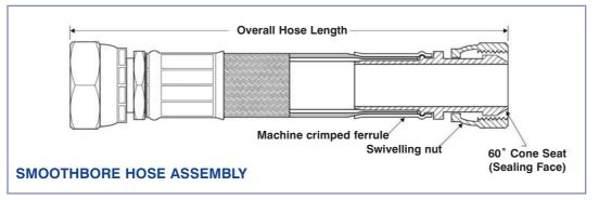
Standard end fittings are BSP cone or flat seat female unions and BSP Taper or NPT fixed males, available in zinc plated mild steel or AISI 316 stainless steel. Other types of end fittings available include stainless steel NPT Fixed Female fittings, JIC fittings, Tube Fittings, standpipes, weld-on fittings, and many others.
