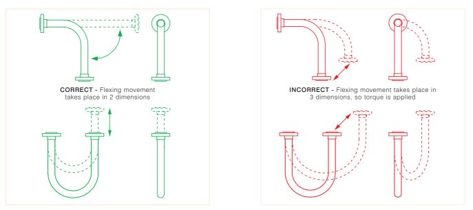
Both Corroflon and Bioflex hose have good resistance to a small level of torque, much better resistance that rubber or SS hose types, but it is still the best practice to take whatever steps are necessary to eliminate torque. If in doubt, consult Aflex Hose.
